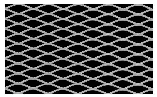
LW Pitch:30.48mmStrand Width:2.00mmSW Pitch:10.00mmThickness:1.50mmWeight:4.71 kg / m2Open Area:60%
